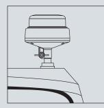
Socket pipe with screw attachment
