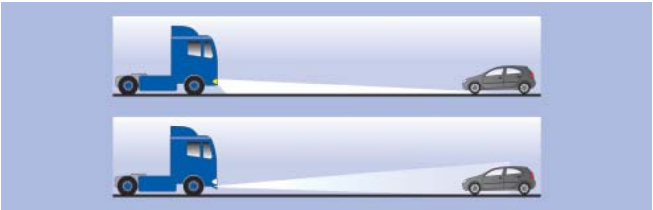
Fig.: Comparison of the two systems: low beam and daytime running light
