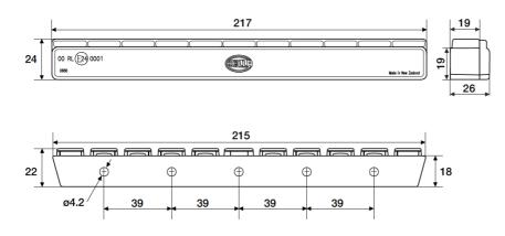
12 LEDs are used as light sources with a power consumption of 2 watts per lamp. They usually last over the lifetime of the vehicle. The LEDs are integral components of the lights and therefore do not have to be replaced. 12 precision lens systems distribute the light emitted from the LEDs in accordance with statutory requirements. The lens made of
