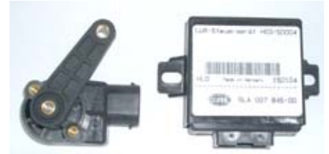
Inductive axle sensor with external control unit
