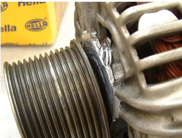
Damaged alternator housing due to worn bearing
