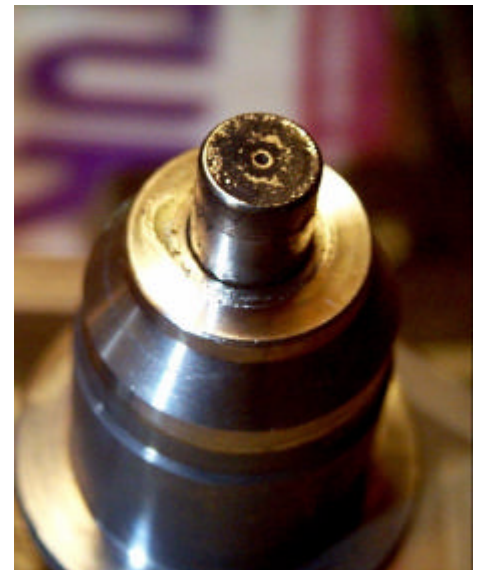
Soiled Injector tip/hole
