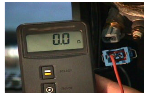
Resistance of the sensor plug to ECU
