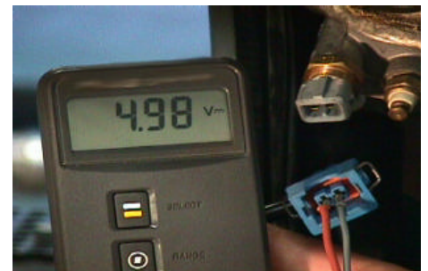
Tension supply at the sensor plug
