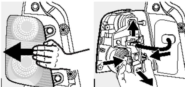
**Important note:** In the case of vehicles built up to 10/06, the ignition key has to be removed from the ignition lock once and then inserted again after bulb replacement, so that the bulb control system can be restarted and the new bulb detected. In the case of vehicles from model year 10/06 onwards, the procedure of removing and inserting the key after bulb replacement is no longer required.
