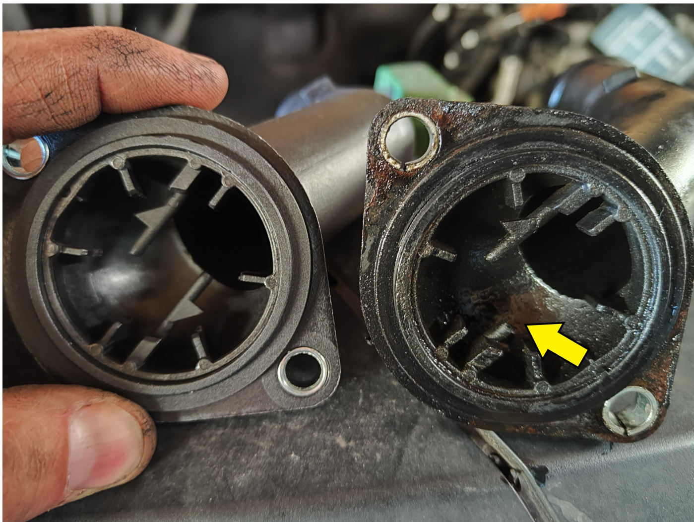
Plastic guide for T5 coolant flange
