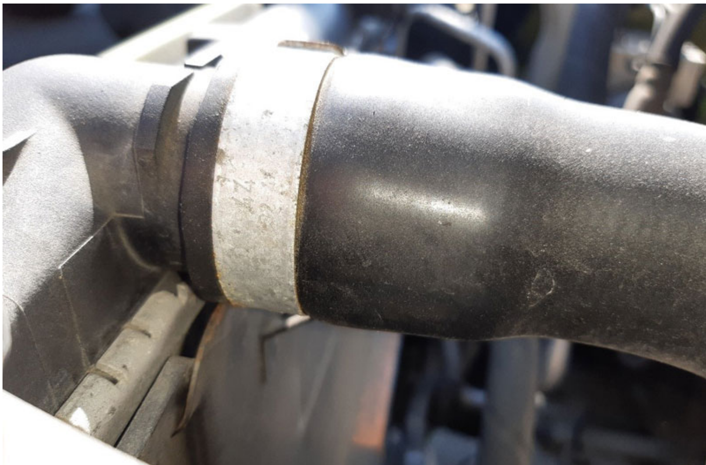
Cooling water hose on the radiator
