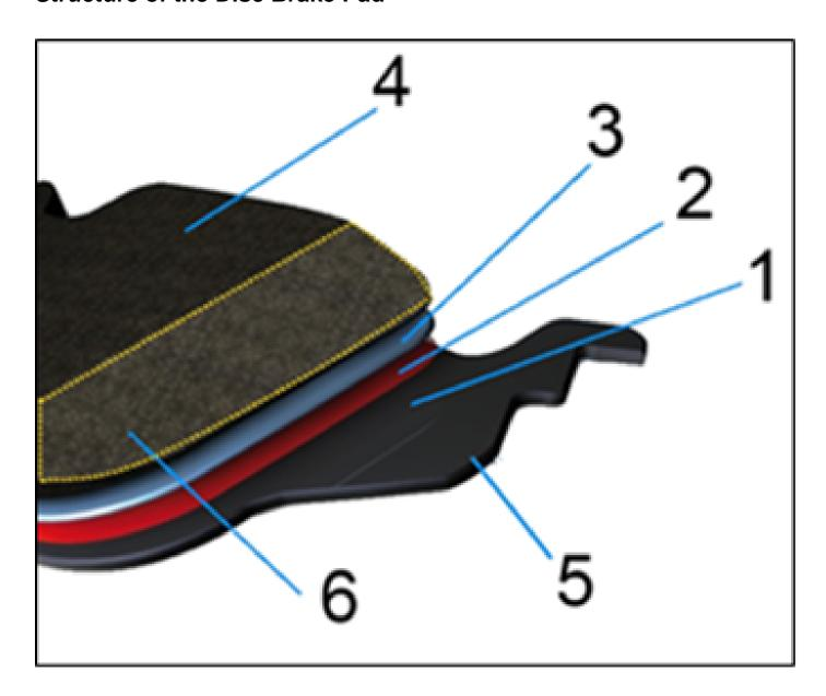
The brake pad has a layered, sandwich-like structure (see diagram).
