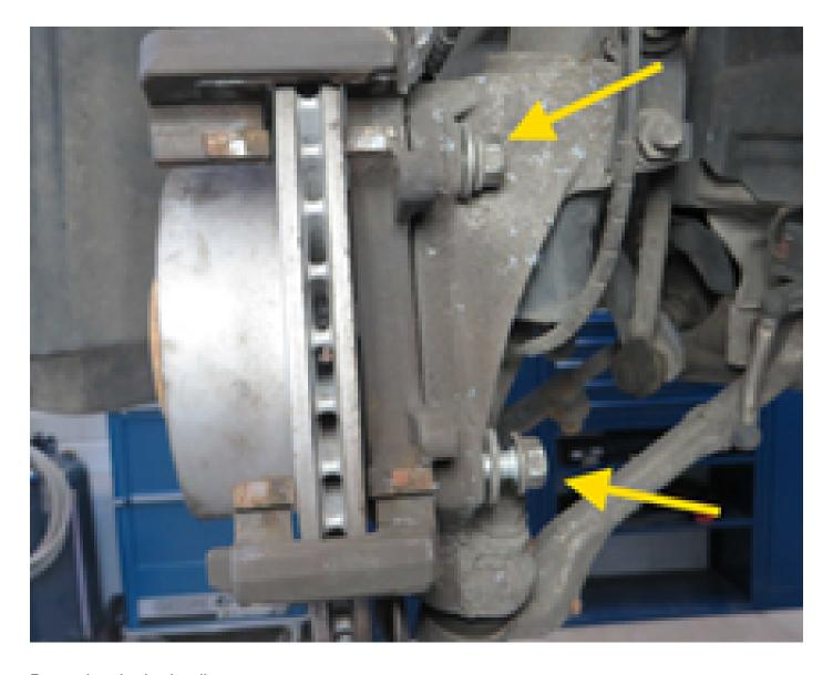
Removing the brake disc
