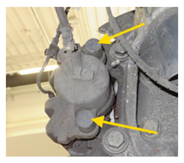
Undo and remove the two fastening screws (guide bolts).
