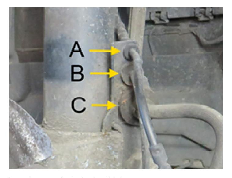
Remove the two protective plugs from the guide bolts.
