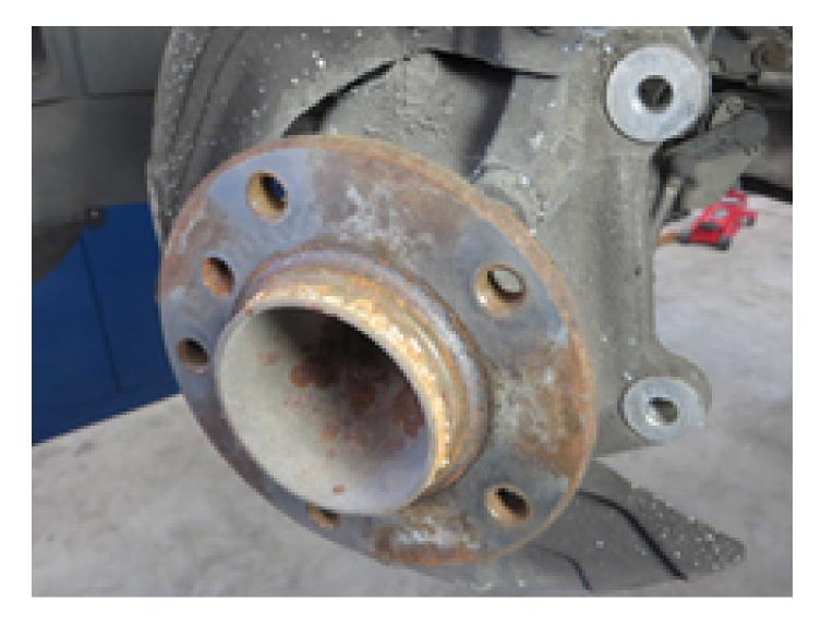
Clean the contact surface of the wheel hub with a suitable tool.
