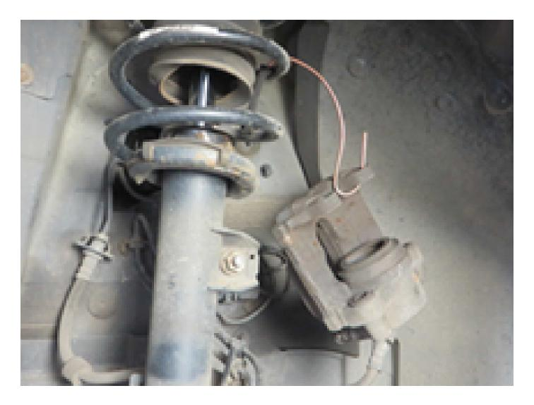
Loosen and unscrew the two fastening screws of the brake caliper carrier.
