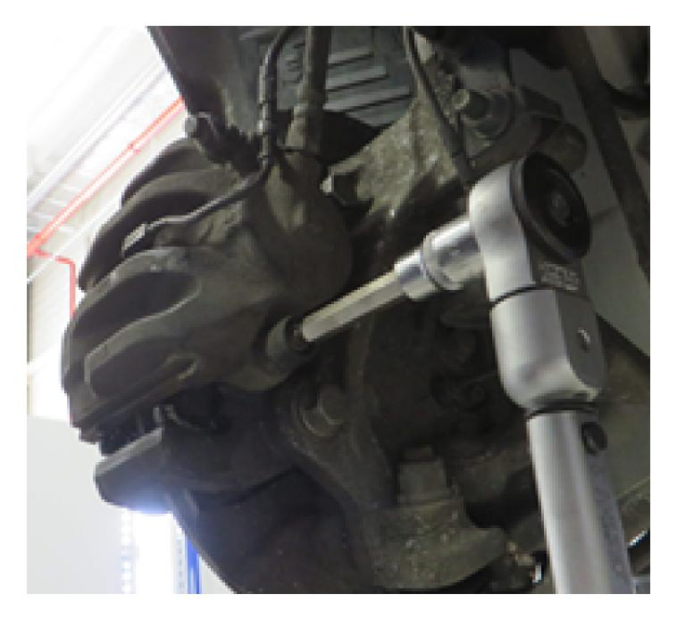
Install and connect a new brake pad wear indicator.
