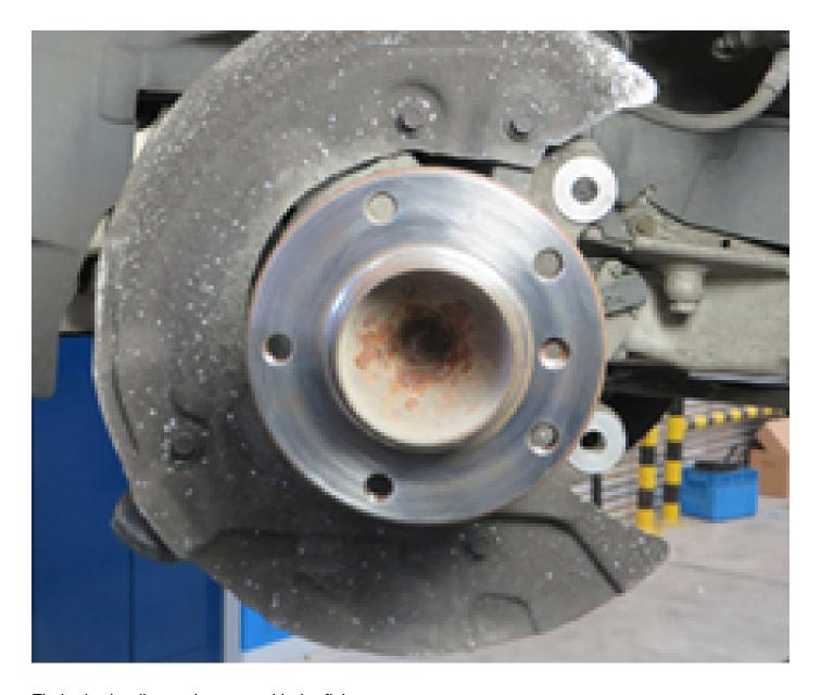
Fit the brake disc and secure with the fixing screw.
