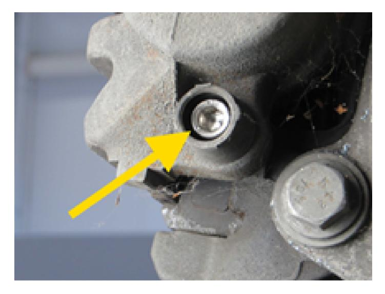
Remove the brake caliper from the brake caliper carrier.
