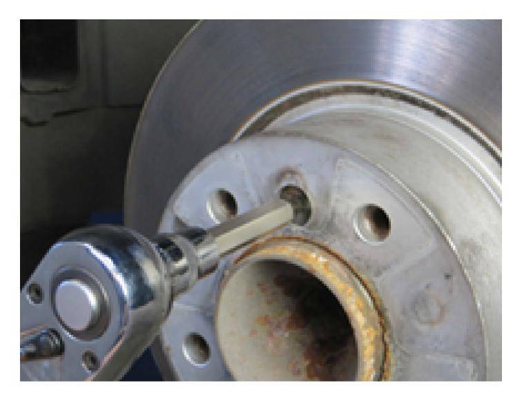
Prepare the brake caliper carrier for installation.
