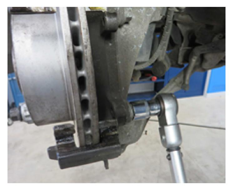
Then apply a thin layer of non-conductive and metal-free brake paste to the cleaned contact surfaces on the caliper carrier.
