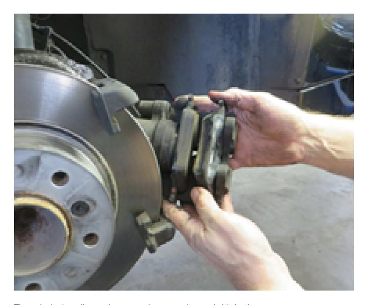
Tie up the brake caliper to the suspension strut using a suitable hook.
