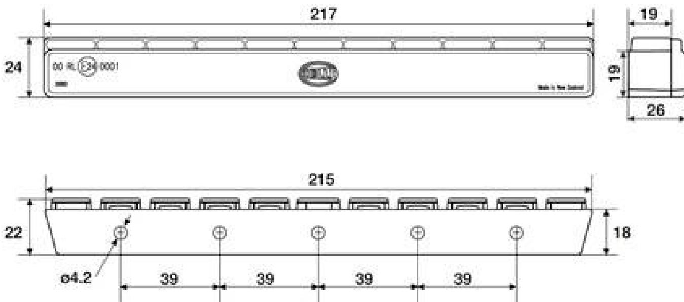
12 LEDs are used as light sources with a power consumption of 2 watts per lamp. They usually last over the lifetime of the vehicle. The LEDs are integral components of the lights and therefore do not have to be replaced. 12 precision lens systems distribute the light emitted from the LEDs in accordance with statutory requirements. The lens made of transparent nylon in the Swiss Grilamid® technology provides high impact resistance and is resistant to UV radiation and chemicals.
