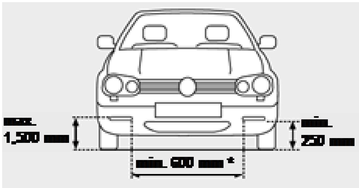
\* On vehicles with a width < 1,300 mm, the distance must be at least 400 mm.
