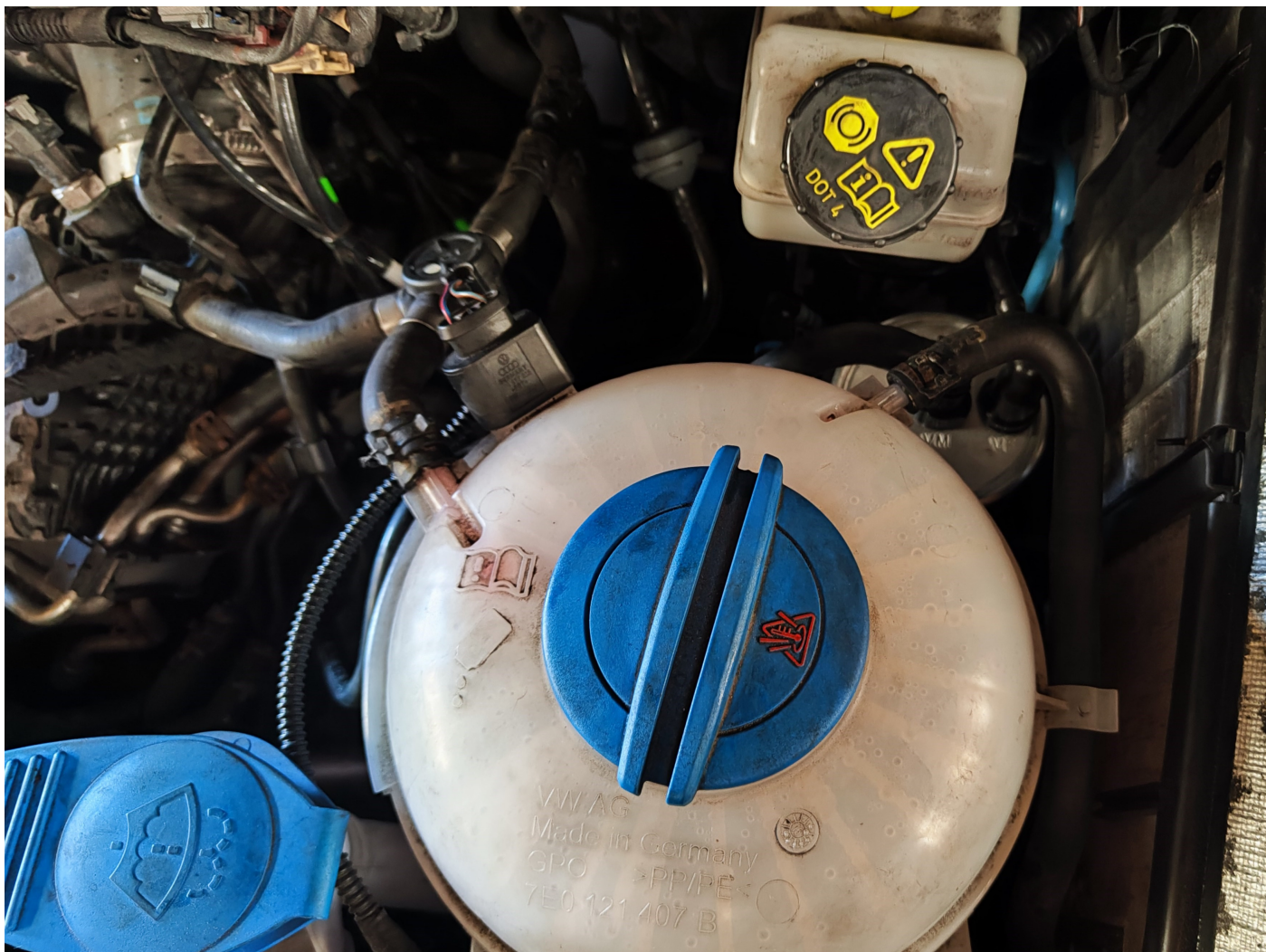
Expansion tank T6
