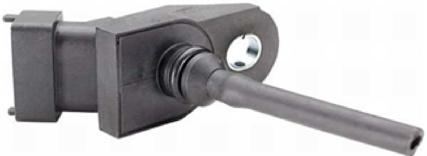
Technical note for the atmospheric pressure altitude sensor: In order to prevent an overrich fuel-air mixture, the injection time is reduced as the sensor voltage increases.
