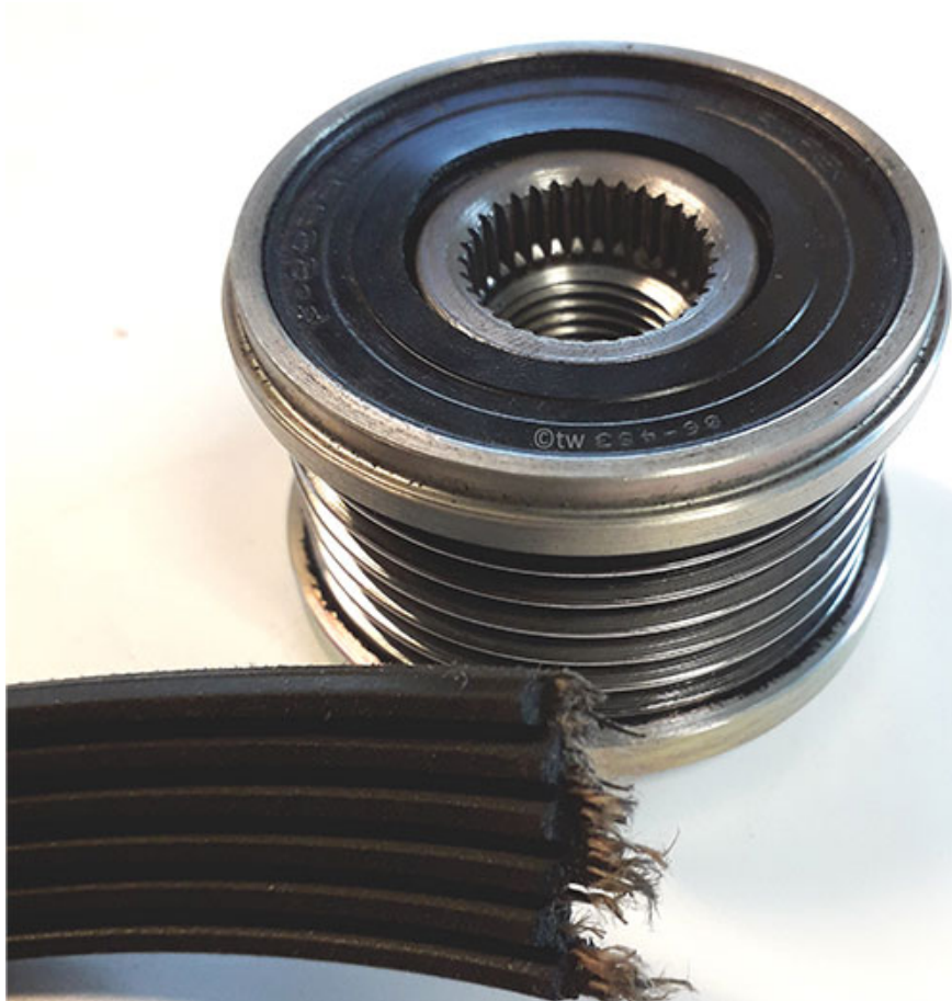
Defective overrunning alternator pulley with torn V-ribbed belt
