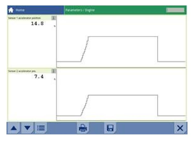
Example: parameter display in mega macs 66 diagnostic unit. Error-free signal curve following confirmation of accelerator pedal sensor
