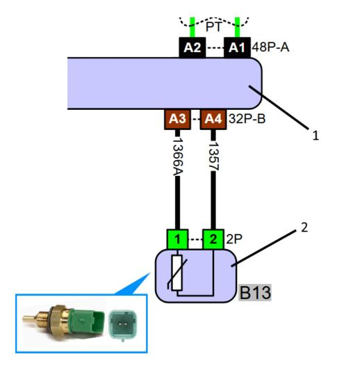
Peugeot circuit diagram Caption: 1: Engine control unit 2: Coolant temperature sensor
