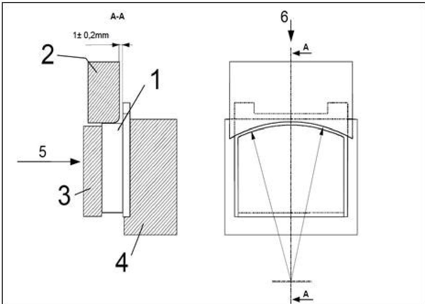
The brake lining (1) is placed in a support apparatus (4) and held there with a counter bracket (3) under slight pressure.
