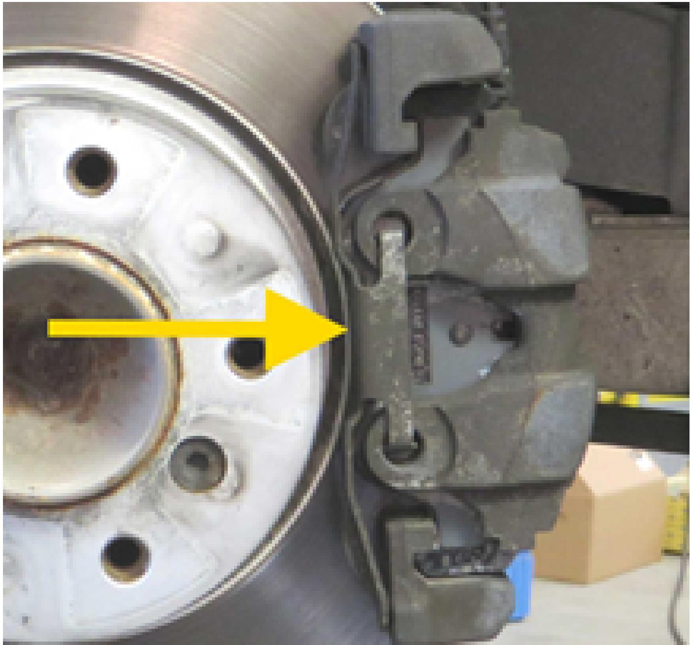
Unclip the wiring harness of the brake pad wear indicator.
