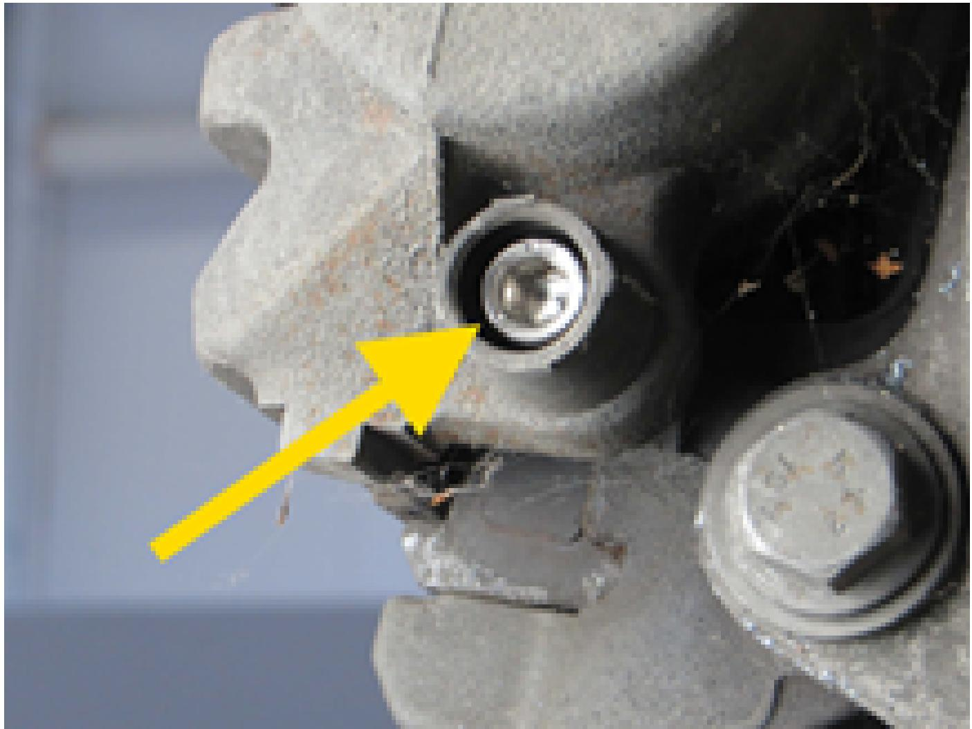
Remove the brake calliper from the brake calliper carrier.
