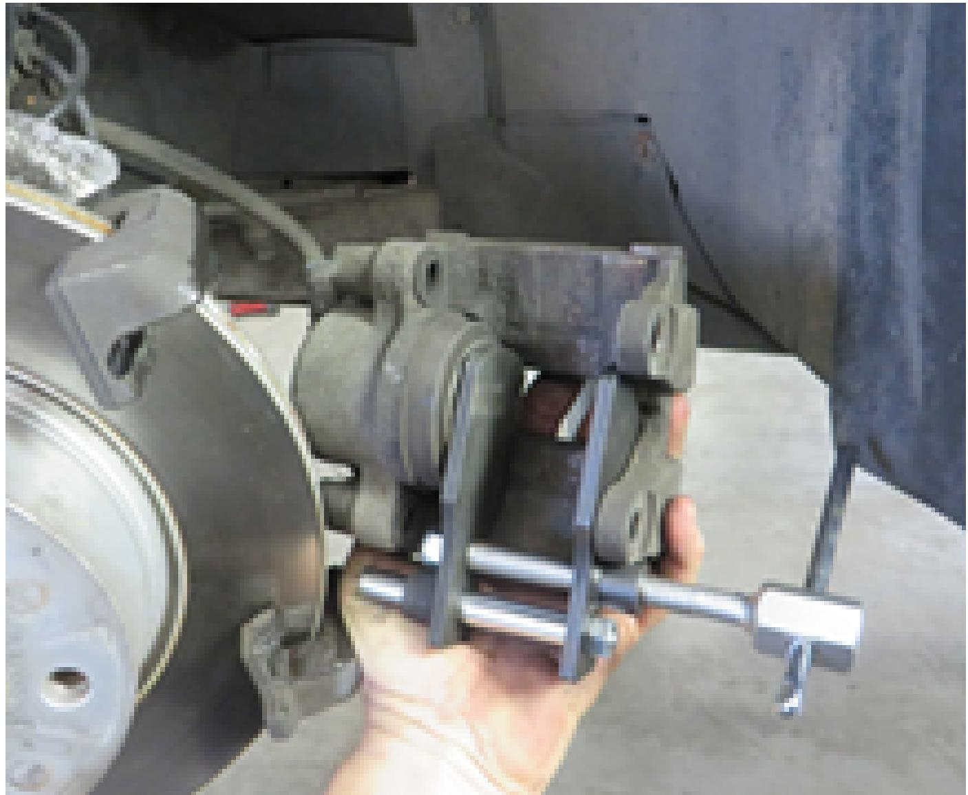
Clean the brake calliper with brake cleaner.
