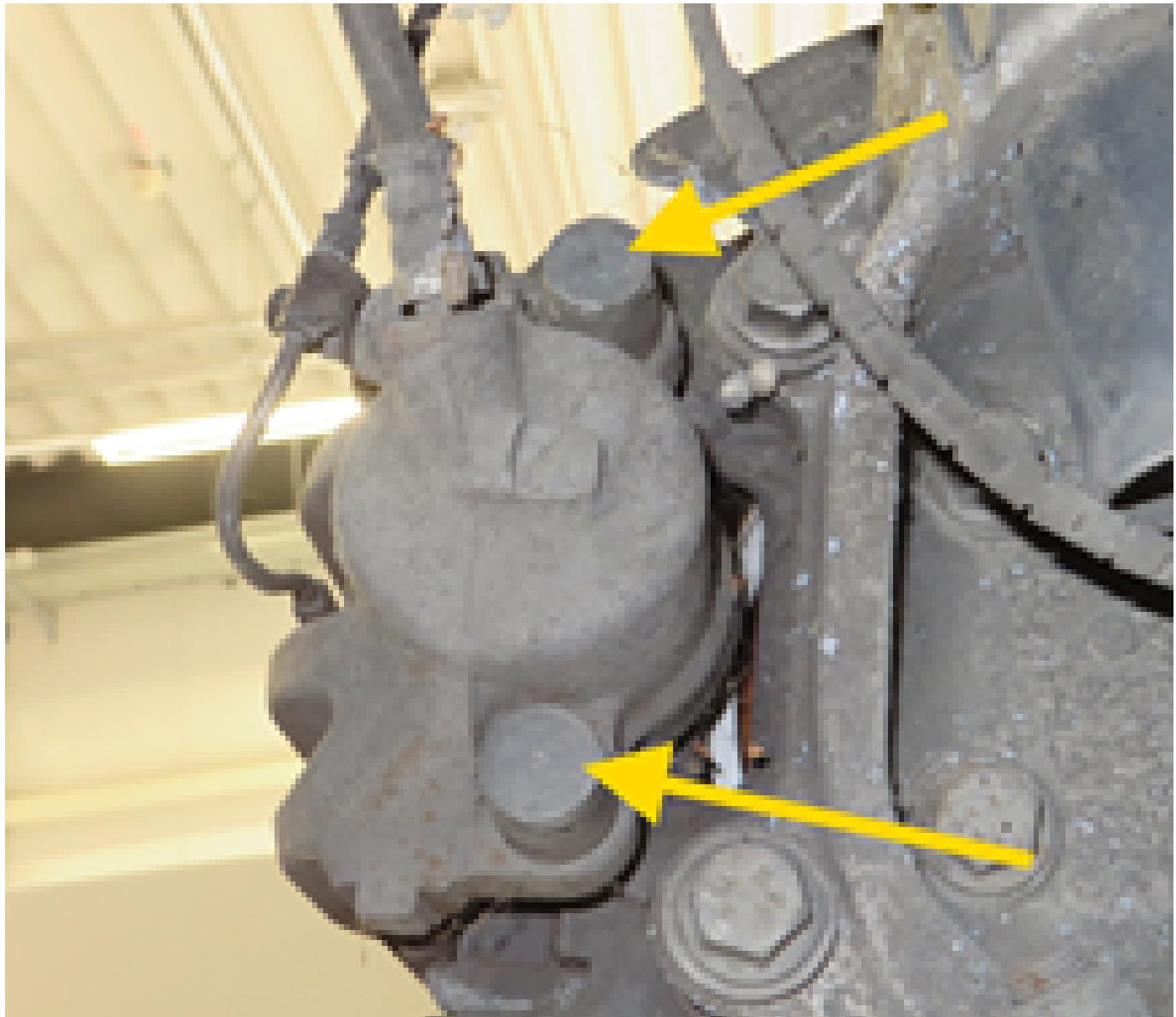
Undo and remove the two fastening screws (guide bolts).
