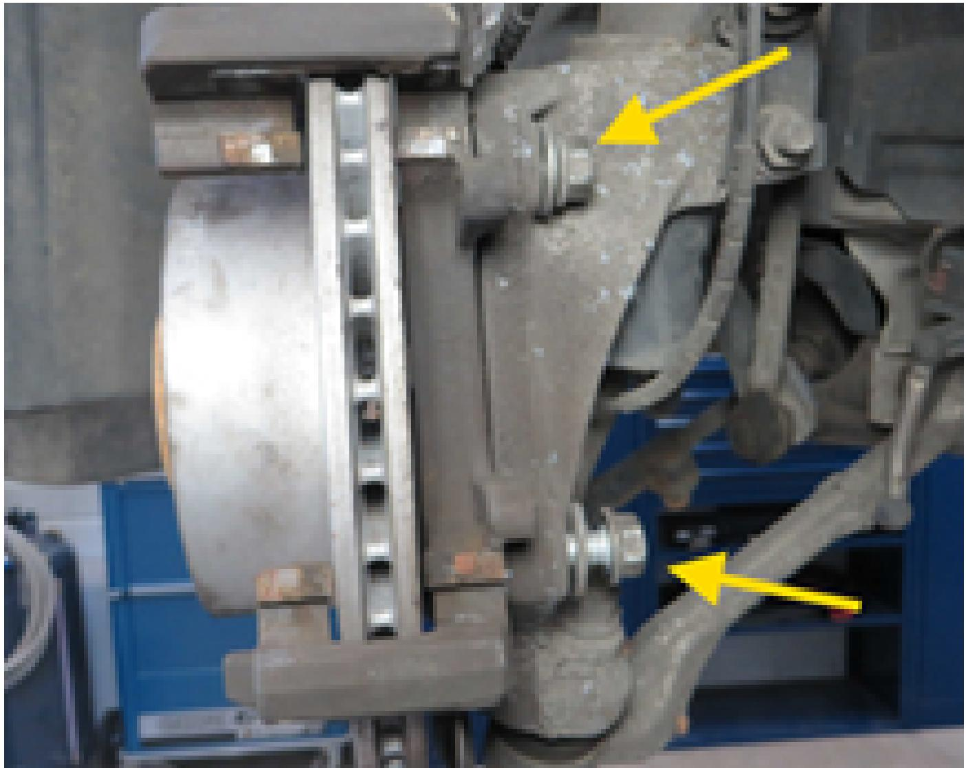
Removing the brake disc
