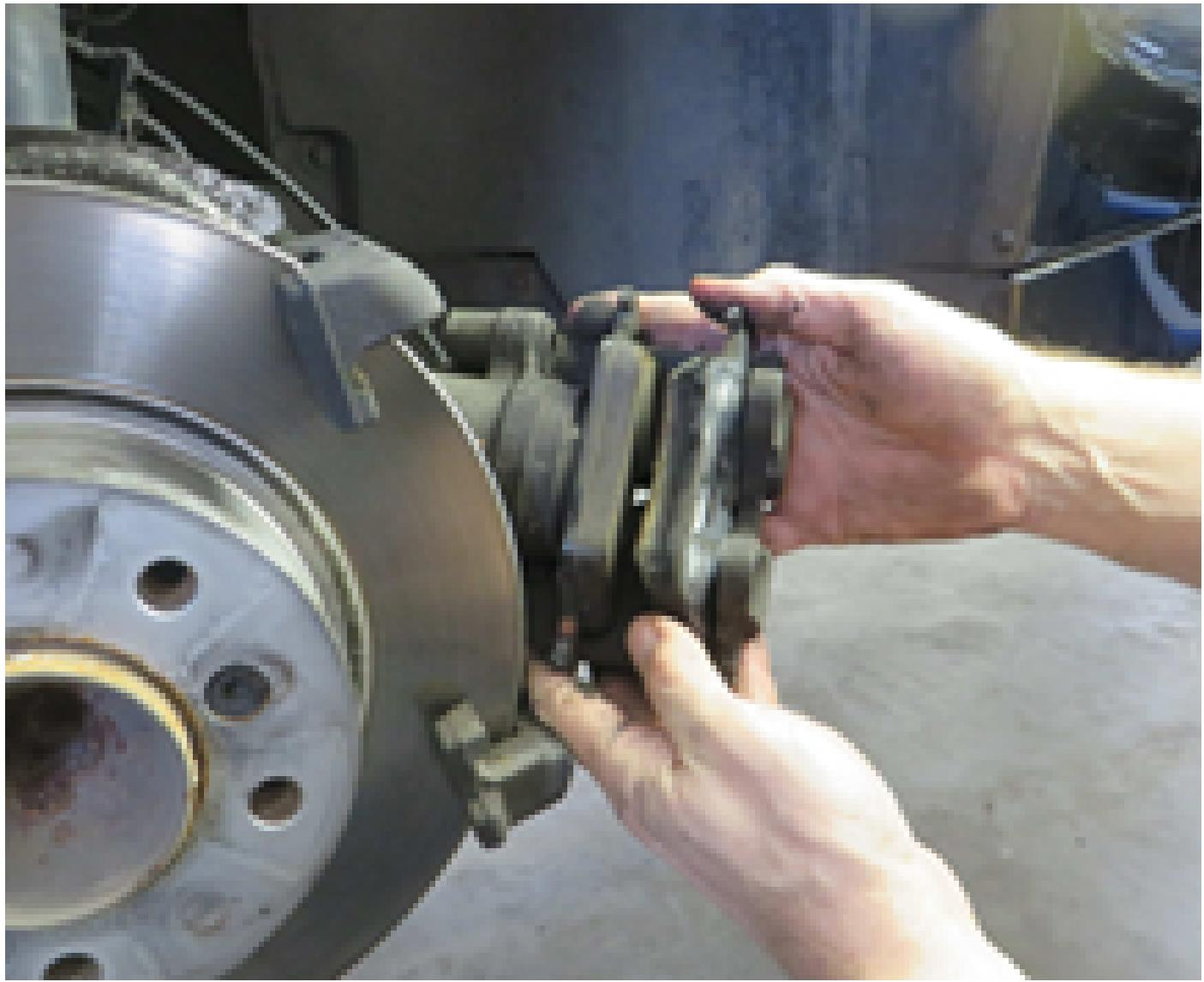
Tie up the brake calliper to the suspension strut using a suitable hook.
