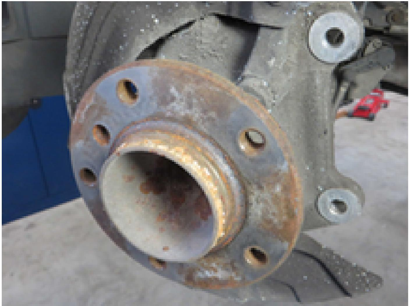
Clean the contact surface of the wheel hub with a suitable tool.
