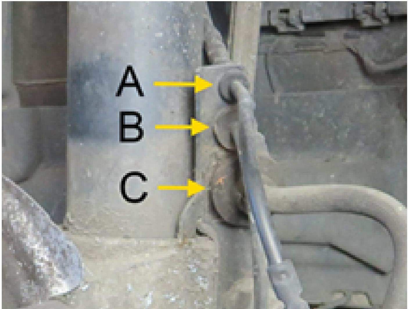
Remove the two protective plugs from the guide bolts.
