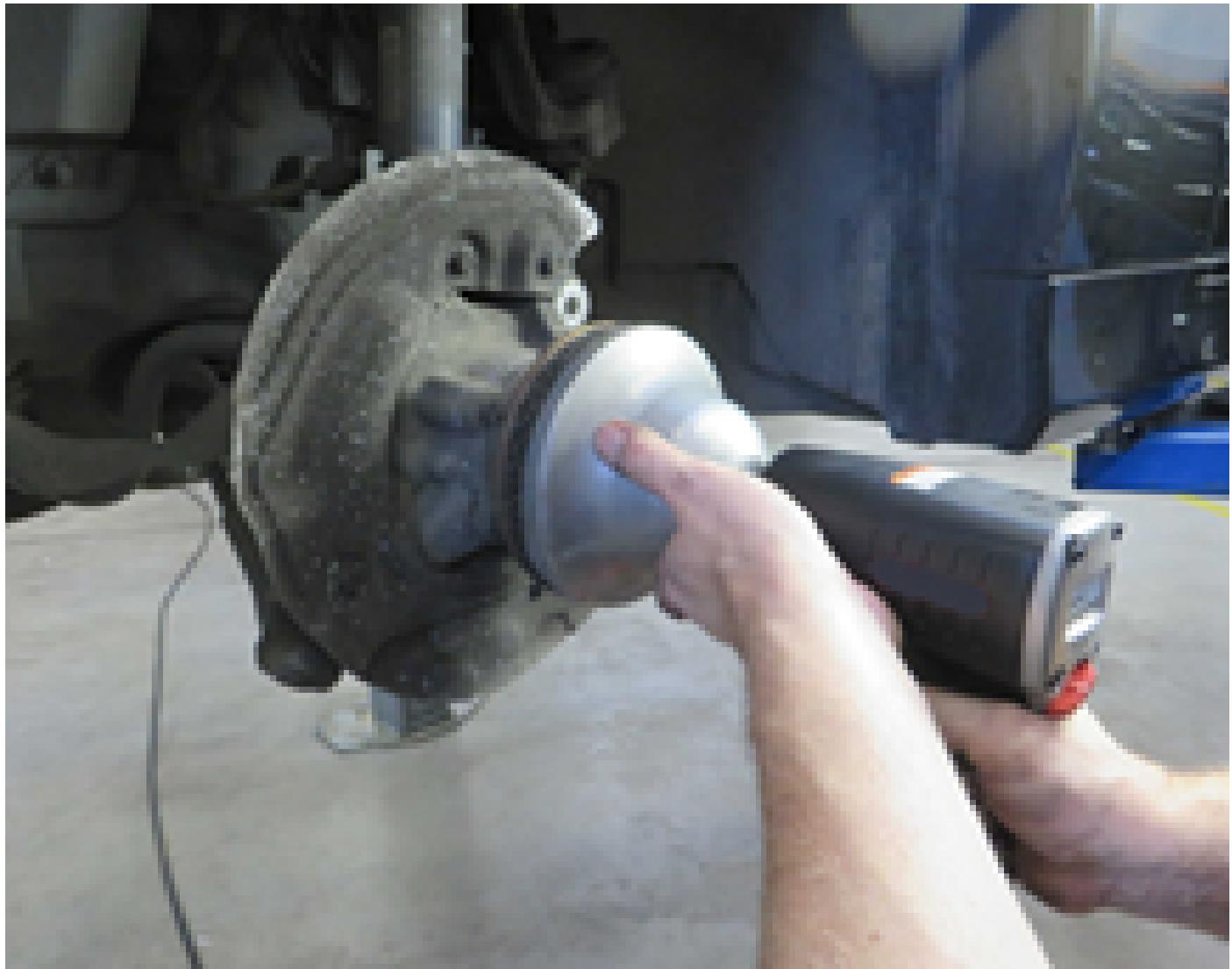
The contact surface of the wheel hub must be undamaged, rust-free, clean and metallically bright. In order to protect against corrosion, spray the contact surface with a thin layer of spray oil and wipe with a lint-free cloth.
