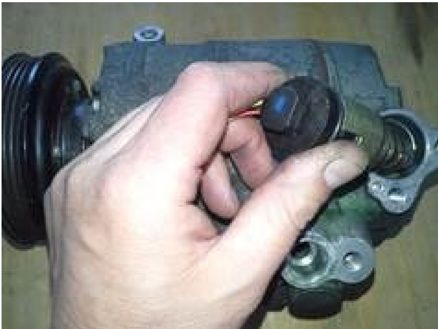
The figure shows an example of compressor with an electronically actuated pressure control valve
