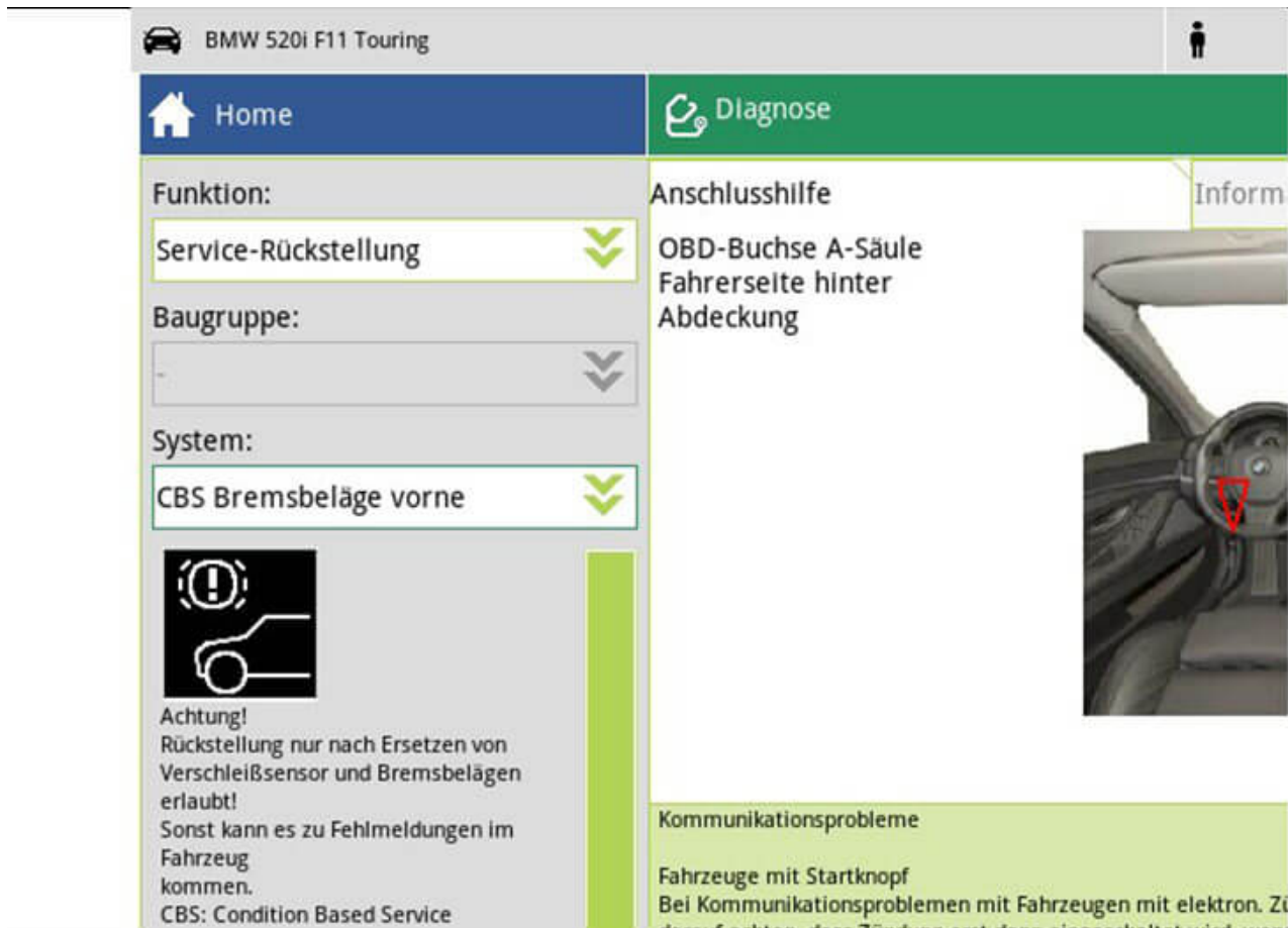
CBS reset with the diagnostic device
