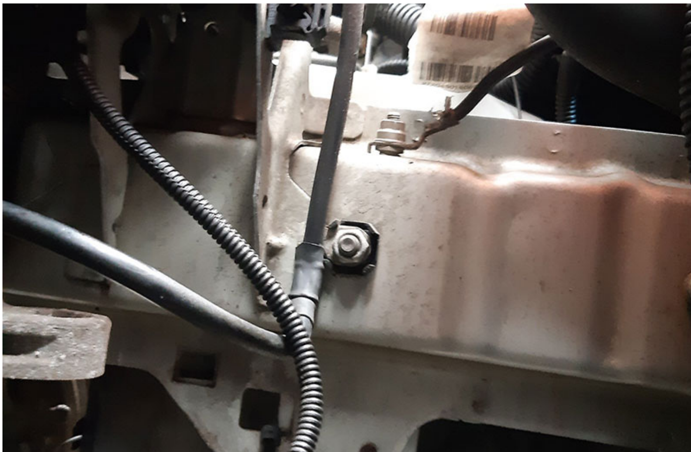
Fiat Grande Punto - engine does not start: Check ground connection
