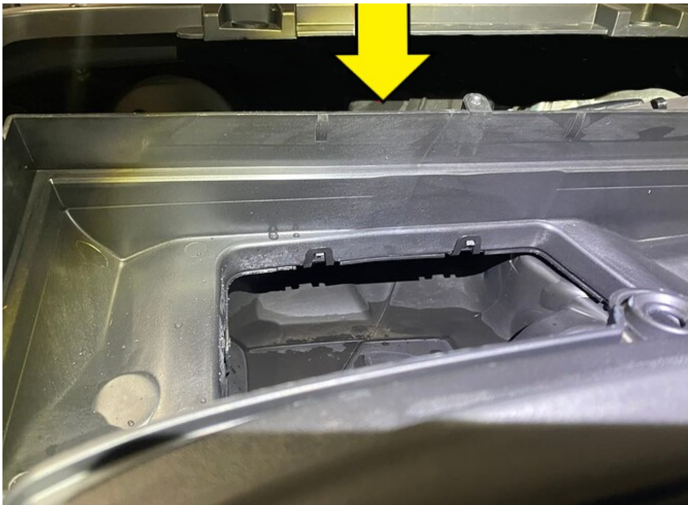
Sealing the ventilation box of the cabin air filter
