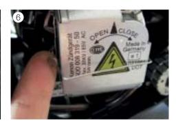
■ Loosen the safety clamp on the ignition module (see Fig. 6).
