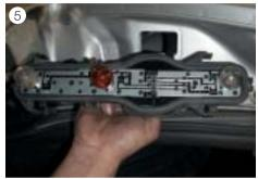
■ Replace the respective bulb in the bulb carrier (see Fig. 5, turned through 90°).
