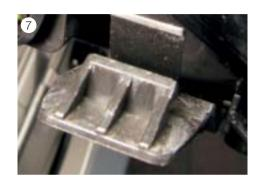
Refit all the removed parts in reverse order. When inserting the headlight make sure that the bottom two headlight brackets (see Fig. 7) have been locked in place properly on the body again.
