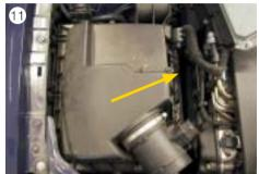
Pull the air filter box (diagonally upwards) out of the guides (see Fig. 11). During this, the hose will also be pulled off the crankcase breather (see Fig. 12).
