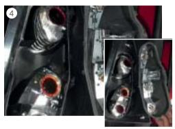
■ Press a rubber wedge carefully between body and lamp until the ball elements become loose from their brackets (see Fig. 3).
