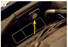
■ Unscrew the fastening screw of the air filter box (see Fig. 5).
