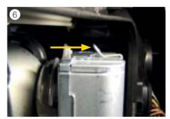
■ Press the safety clamp for the supply cable towards the rear (see Fig. 6).
