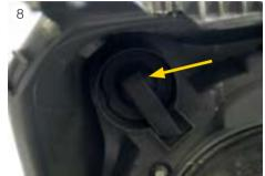
■ Pull the rubber cap off the parking light, take the socket with the bulb out of the reflector and replace the bulb (see Fig. 8).
