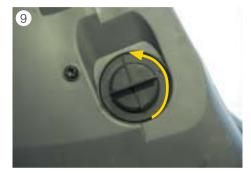
■ Turn the indicator bulb socket base anticlockwise as far as it will go and remove it from the headlight together with the bulb (see Fig. 9).
