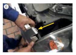
■ Pull the front trim forwards slightly and remove the headlight from the body (see Fig. 6).
