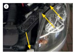
■ Unscrew the fastening screws (Torx 30) on the headlight (see Fig. 4).
