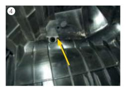
■ Pull the rubber bolt in the lower part of the air filter box upwards and out (see Fig. 4).
