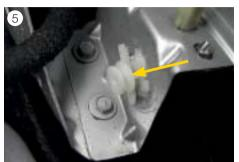
■ The headlight now has to be pulled forwards sharply to release it from an additional guide. This is on the bottom (wing side) of the headlight (see Fig. 5).
