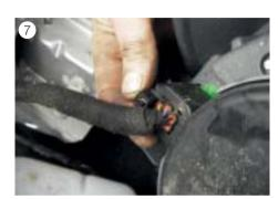
■ Loosen the plug connection and pull the plug off the headlight (see Fig. 7).
