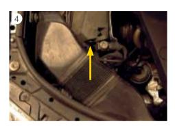
■ Pull the air channel up and off the air filter box (see Fig. 4).
