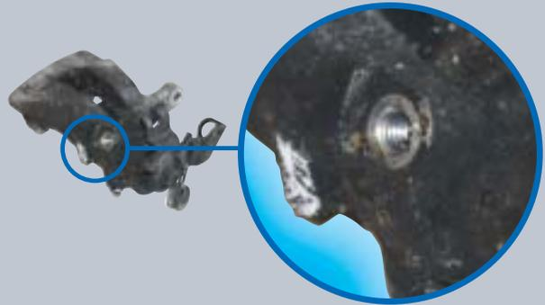
Guide bushing damaged
