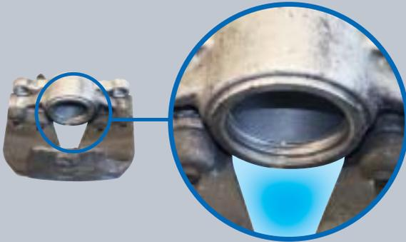
Handbrake activation lever mechanism missing
