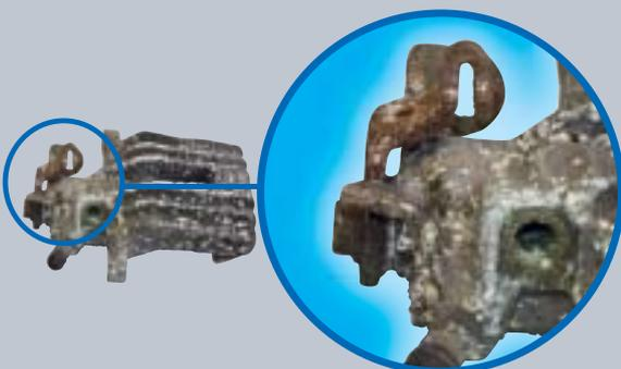
Internal oxidation. Brake piston seized up
