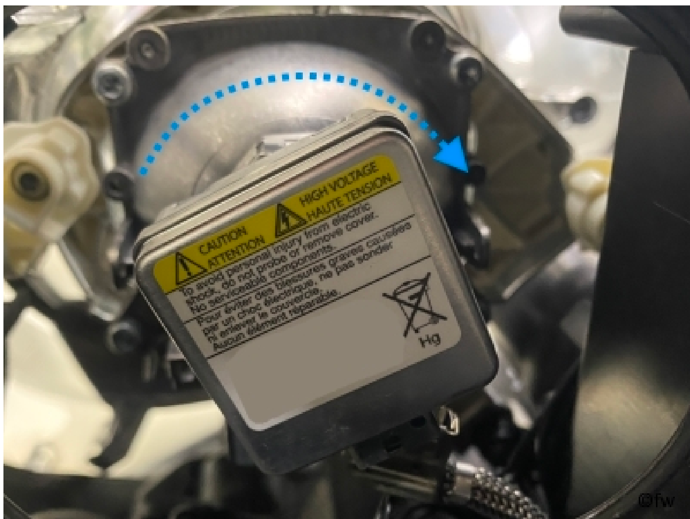
Rear view of the Mini R57 light source
