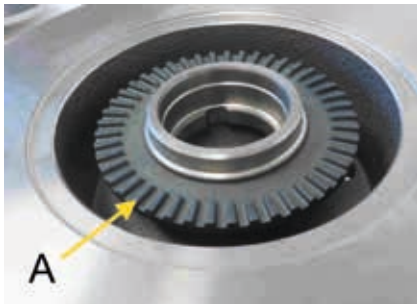
Brake disc without wheel bearing but with permanently fixed impulse ring and vertically positioned toothed segments (A).
