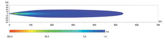
The light distibution shows 2 high-beam headlamps each in function.
