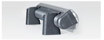
Angle adjustment: 20° downward and 30°upward when mounted upright. (Tighten mounting nuts to hold at the set tilt angle)
