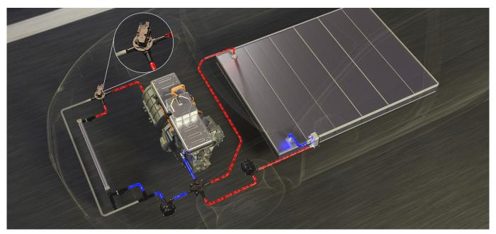
Cooling circuits in a wide range of vehicle segments
