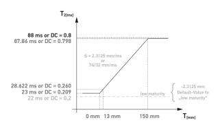
$T_2/T$  = DC = 0.2 :  $T_2$  = 22 ms => Unreliable signal (Level output -2.3125 mm)
