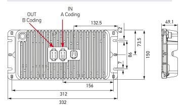
\* With 1-channel operation only the left pin is used IN/OUT, the right one has no function. See page 4 for part numbers.
