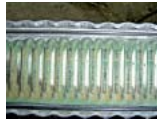
Limescale deposits due to the use of pure water (without coolant).
