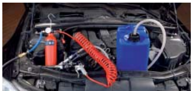
Flushing with flushing solution
