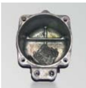
Abrasion with compressor damage
