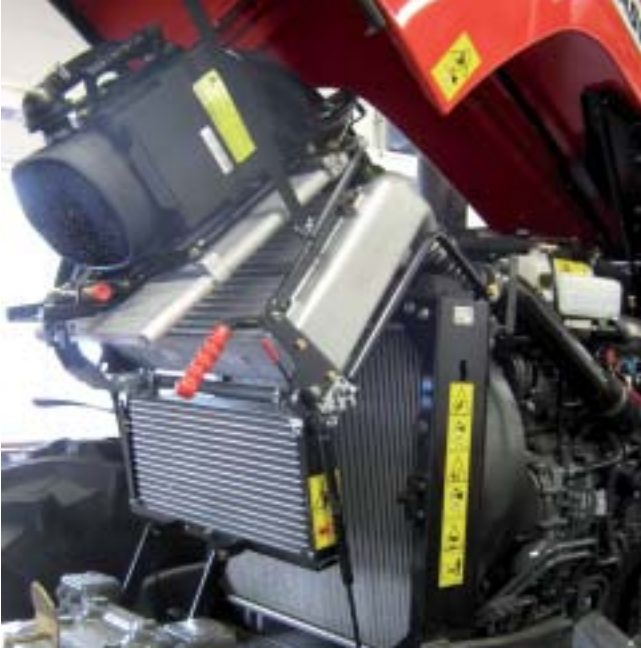
Cooling system today
