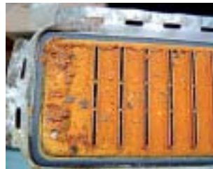
Deposits due to a discharge of oil are caused by engine oil entering the coolant circuit as a result of a damaged cylinder head gasket.
