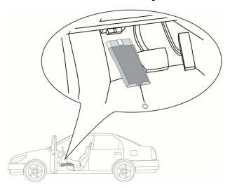
1. Insert the DT VCI into the vehicle's diagnostic connector.
