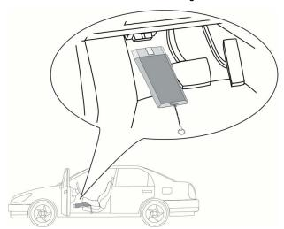
2. Insert the DT VCI into the vehicle's diagnostic connector.
