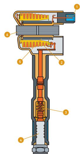
In systems with single-spark ignition coils, one ignition coil with a primary and secondary winding is assigned to each cylinder. These ignition coils are usually installed directly at the cylinder head, above the spark plug.
