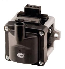
The primary circuit receives its voltage supply through terminal 15. The contact breaker is connected to terminal 1 of the ignition coil, and supplies the primary winding with ground. The high-voltage wire of the ignition distributor is connected to terminal 4. Whereas conventional ignition coils are still being used with older vehicles, ignition coils with integrated electronic control units are now used in vehicles that are equipped with a transistor ignition.
