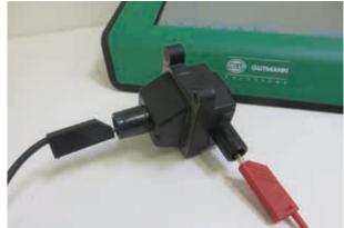
To measure the secondary coil, measure the test probes directly at the high-voltage outputs of the ignition coil.
