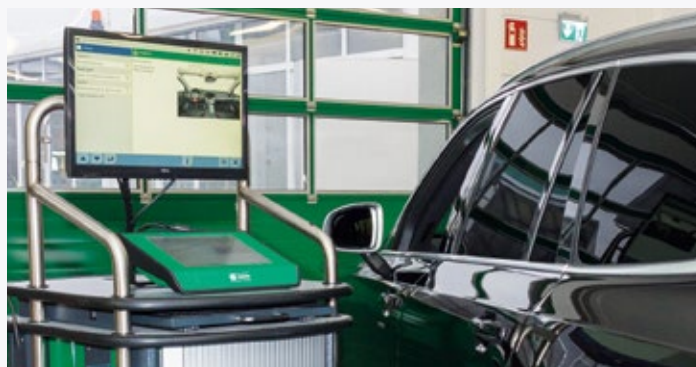
Data is transferred to cars such as the latest BMW 5 Series and Volvo XC90 via DoIP
