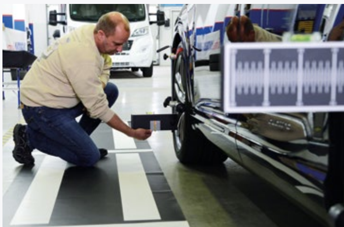
The Wheel Sensor Control enables a fast, trouble-free check of a vehicle's tracking
