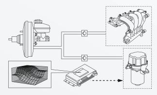
This variant operates without a pressure sensor and is controlled via induction pipe pressure characteristic maps deposited in the engine control unit. Induction pipe pressure is calculated from the input variables, the engine speed, the engine load, the throttle valve position and the stop-lamp switch.
