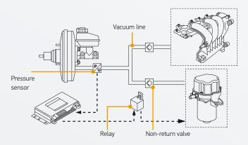
In the case of the regulated variant, a pressure sensor is installed in the vacuum line to the brake booster. The pressure sensor permanently registers the actual pressure in the system and conveys this value to a higher-level electronic control unit (e. g. an engine control unit).
