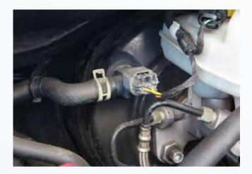
The diagnostics will now be illustrated by using the example of an Opel Cascada 1.4i 16V Turbo, model year 2013 with a mega macs 77 diagnostic unit. This example, however, also covers vehicle models which are identical in construction. This vehicle with a turbocharger and STOP-START system has a HELLA UP28 vacuum pump with a pressure sensor on the brake booster installed.
