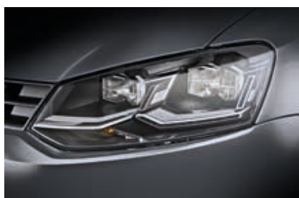
Small car / VW Polo (2014): LED front headlamp with reflector system for low beam and high beam
