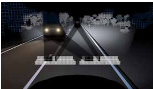
Glare-free high beam light due to targeted masking of individual LED modules
