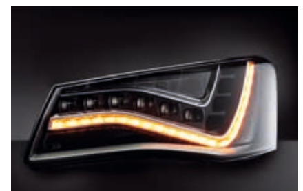
Stylish design and light signature options due to LED technology (example: Audi A8 full LED headlamp)
