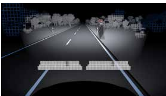
Traffic sign detection with reduction in glare affecting the driver's own vehicle
