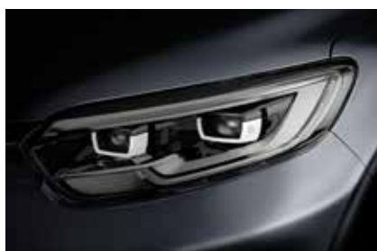
Compact class / Renault Kadjar (2015): LED front headlamp with HELLA mono- LED modules for low beam and high beam
