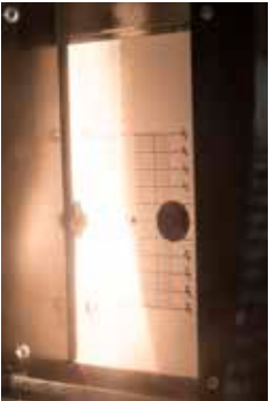
Low beam measurement for the Mercedes W 202 left-hand drive vehicle BEFORE masking: Normal asymmetrical light distribution
