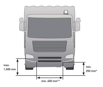
Legislation permits different attachment variations. However, the distances and beam angles to be adhered to are specified.
