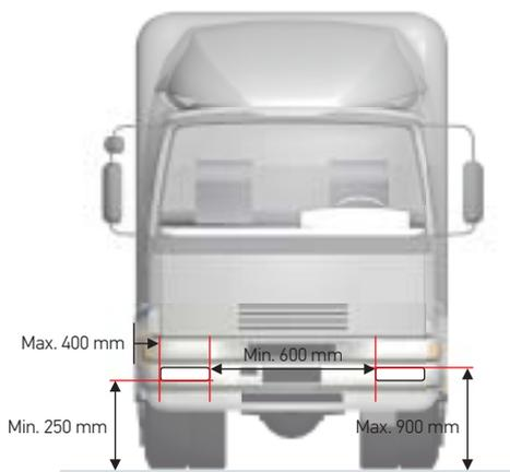
\* An exception is only possible if the vehicle geometry does not make standard installation possible.
