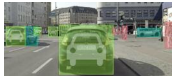
AI based vulnerable road user and automatic emergency braking in low cost NCAP camera
