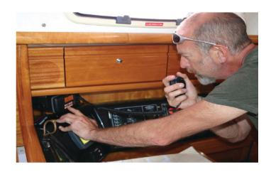
All active electronic devices, including LED products, create some degree of EMI. The danger comes when this interference occurs in the frequency range between **156 MHz and 165 MHz**, used by **marine VHF and AIS systems**. This can potentially compromise communication, with major operational consequences posing a serious safety risk.
