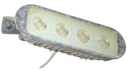
A powder coated aluminum floodlight with housing degradation
