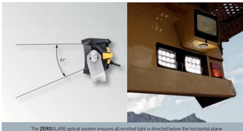
The ZEROGLARE optical system ensures all emitted light is directed below the horizontal plane
