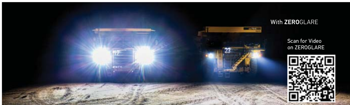
The ZEROGLARE optical system ensures all emitted light is directed below the horizontal plane
