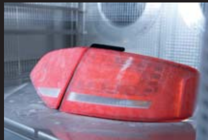
Humidity and cold test
