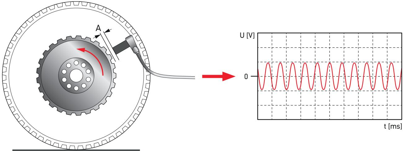
The wheel speed sensors are mounted directly above the pulse wheel connected to the wheel hub. The pole pin, which is surrounded by a winding is connected to a permanent magnet, whose magnetic effect extends to the pole wheel. The rotational movement of the pulse wheel and the associated change of tooth and tooth gap causes a change in the magnetic flux through the pole pin and the winding. This changing magnetic field induces a measurable alternating voltage in the winding.
