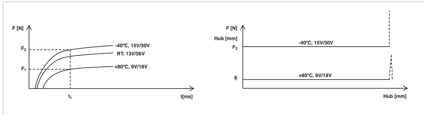
With a controller time of  $t_1$ , the actuator has an actuating force of  $F_1 < F < F_2$ . The constant actuating force on the tappet over the rated stroke depends on the operating voltage and ambient temperature. If the actuator has no load to move over the stroke, the actuator power is converted into a higher actuator speed, resulting in the dynamic impact pulse becoming a multiple of the constant actuating force.
