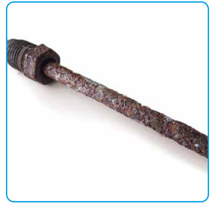
External damage, grizzly raise
