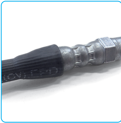
Bubble formation in transition areas Braided hose fitting
