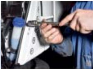
**14** Finally you can fit the finishers equipped with the daytime running light modules back onto the vehicle front-end.
