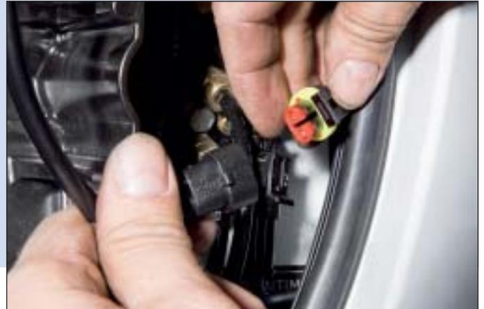
**12** Connect the blue cable (ignition plus, terminal 15, terminal 15 fuse must be connected at the additional slots on the right in the fuse box) with the black cable. The grey cable has to be connected with the aid of butt joints to the position light cable (terminal 58) at the central plug of the headlights (PIN 2, grey-red cable), so that the lights are switched off when the parking light or low beam are switched on.
