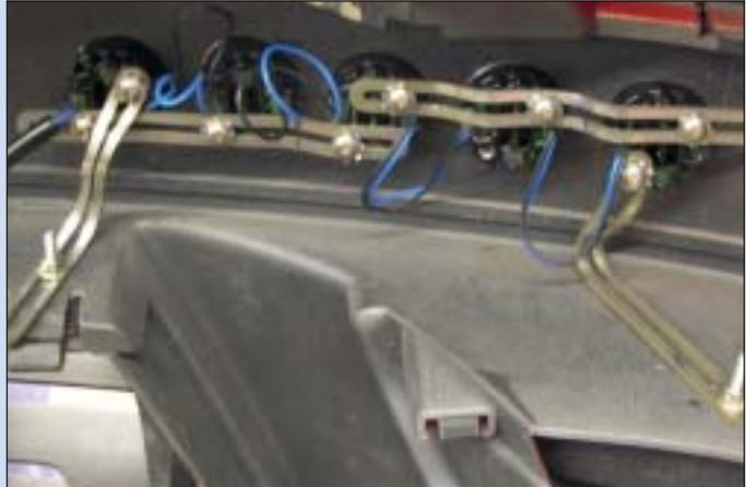
**10** In addition, reattach the removed holder (see step 5) to the finisher. Rivet this in place from the inside, where the LEDs are. Riveting from the outside will prevent the rubber from fitting. Now carry out installation steps 2-10 for the other side, too.
