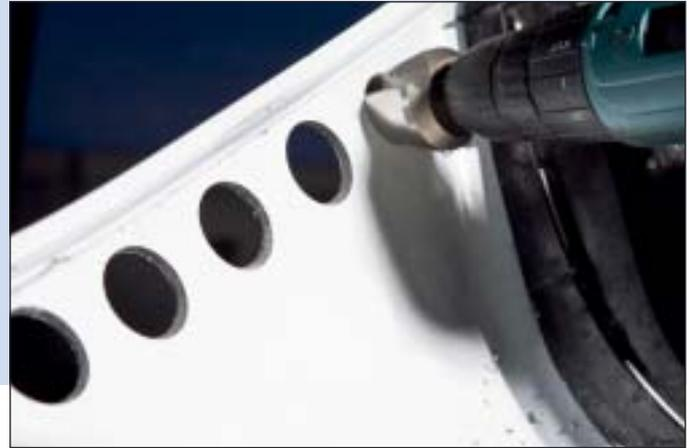
**7** Now you have to deburr the holes by hand using a deburring tool.
