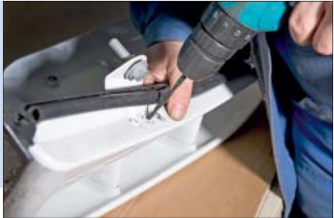
**6** Now drill the holes at the points shown in step 2 in the respective size for the modules (diameter 30 mm).
