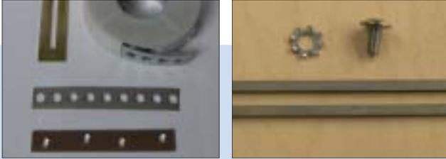
**9** To attach the individual modules to one another, small stainless steel rails that can be adapted easily are the ideal solution (see fig.). Then attach the complete “chain” to the plastic panelling using two holders.
