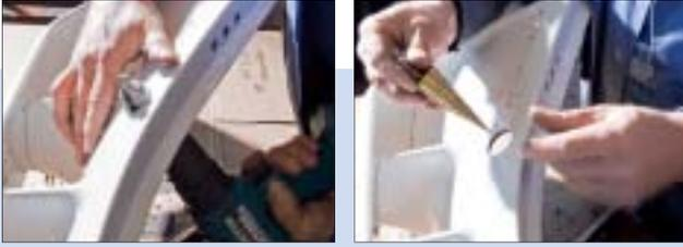
Check the size of the holes at intervals by holding the modules in place. You could drill the holes too big, which would result in a poor appearance. So check the diameter regularly during drilling.
