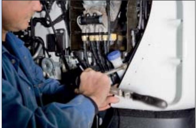
**5** Drill the fastening rivets open and remove the holder with the rubber strip. Now unscrew the holder on the finisher. If you do not do this, it will not be possible to drill the holes for the LED modules.
