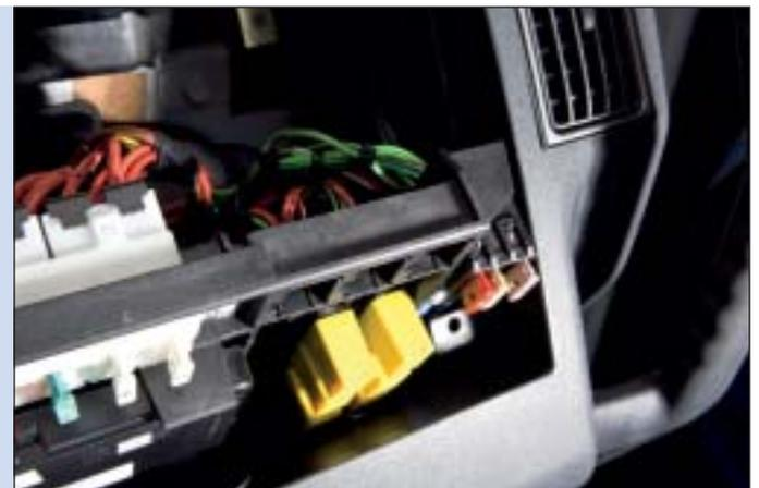
Finally, all you have to do is fix the eyelet of the brown cable to a suitable ground point. Rather than using the LEDayFlex connection cable set, you can also prepare the wiring yourself.
