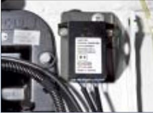
**11** Now fit the control units for the daytime running lights on the left and right in the engine compartment. Then you can connect the cable in the engine compartment with the connection leads on the control units.
