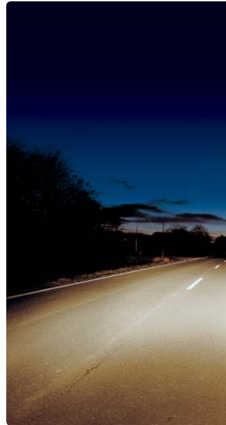
Typical light distribution and color temperature of a headlamp with standard halogen lamps.
